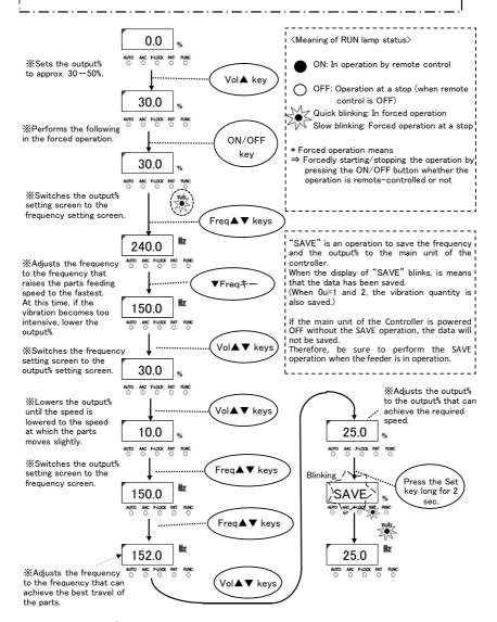
(4)-B When the Vibration Sensor KS-3 is used (When the feedback control is performed in the constant amplitude mode, 0u=1, 2)
