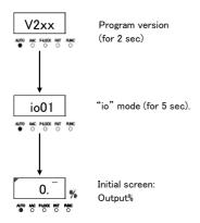
② Switching from the operation mode to the adjustment mode
