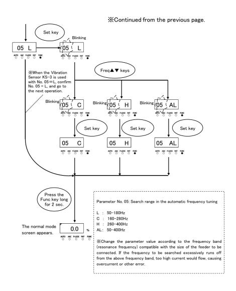
When the Vibration Sensor KS-3 is not used, go to ④-A. When the Vibration Sensor KS-3 is used, go to ④-B.
