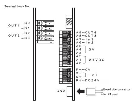
Wiring to the external signal terminal block (screw-less)
