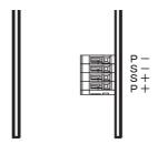
Wiring to the external signal terminal block (screw-less)
