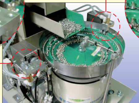
平头螺丝用带分料单元的部品供给系统 Parts feeder system w/escape for countersunk head screws
